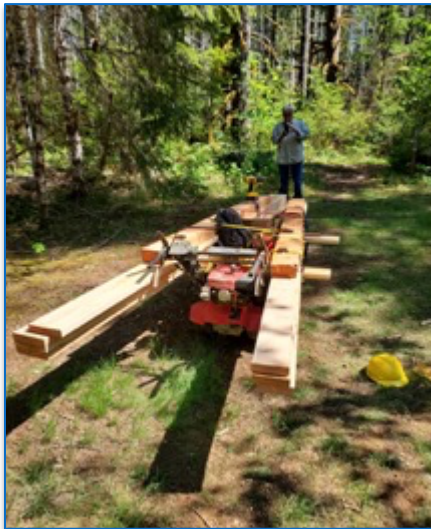
Lumber for repairing bridges was hauled with a motorize tote.
