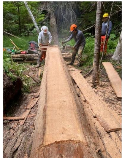
Left: The first time you run the mill down the log, it has to be on the rails you see in the picture. We take off a thin layer first that is discarded. That gives us a flat surface. We are lucky that Paul Hornberger and Mike Bonomo had used this device a lot to make decking for the Slab Camp bridge replacement in 2018. They taught the rest of us how to set it up and use it. We are also lucky that Tom Mix has collected and tended useful but uncommon tools like this for BCH over the years.
